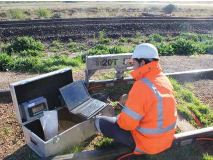
Static point load calibration of TrackWeigh system at Condobolin in NSW.
